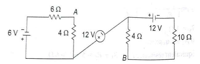
8. a) Find the voltages at node1 and node2 by using node analysis
