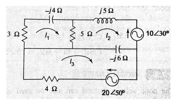
b) find the mesh currents in the given circuit.
