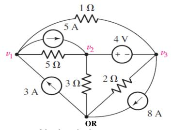
b) Find the h parameters of the given circuit.
